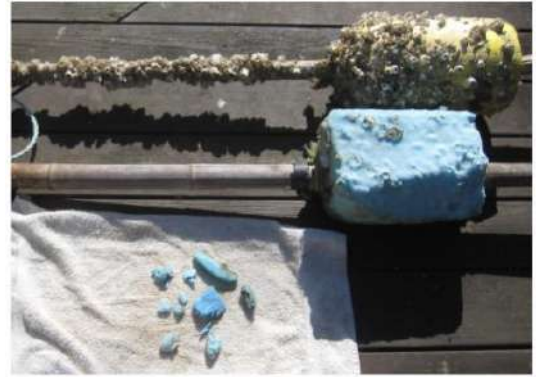
The lower disintegrating blue Styrofoam buoy, and foam crumbles or microplastics ingested by fish and birds directly or through the food web. The upper yellow one is a recent Styrofoam buoy with bamboo pole covered in barnacles.
